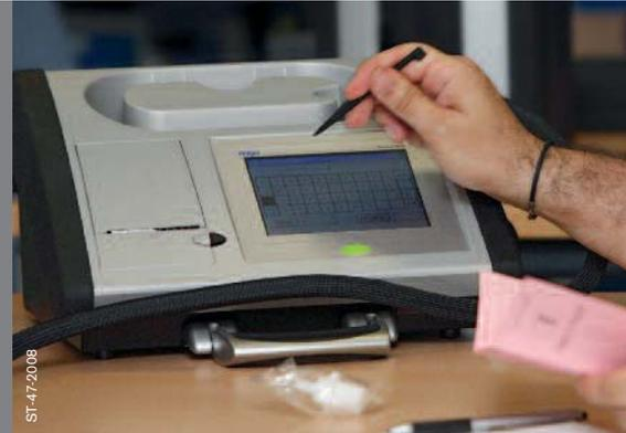
In many countries the results of breath alcohol testing are admissible as evidence in court. Instruments used for these measurements have to fulfil very tight requirements and have to be very reliable. The Dräger Alcotest 9510 represents a new generation of breath alcohol measuring instruments. It is designed to comply with most international regulations for such devices which are besides national regulations especially the requirements defined in OIML R 126-1998.
